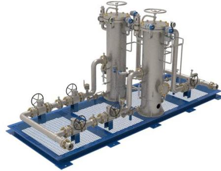
Fuel Gas Conditioning Unit is designed to treat (remove unwanted liquids and solids) the natural gas before delivering to the gas turbine. Fuel Gas Conditioning Unit is also called Fuel Gas Conditioning System because it consists of several types of parts which performs various functions to achieve the required conditions of the natural gas for delivering to the gas turbine.
